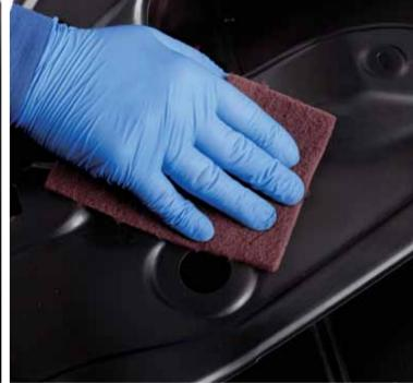
Preparation Of E-Coat & Awkward Areas: Gripspeed Weave Pads, Very Fine (Red) Hand Pads, Rolls, Weave Prep Pads
