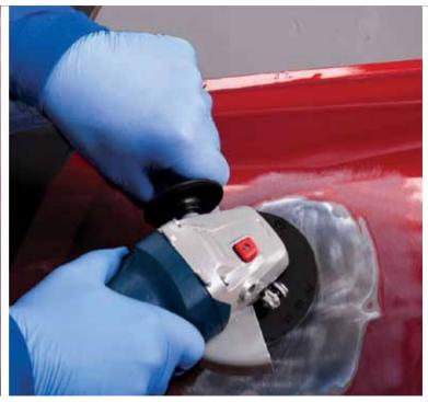
Weld & Stock Removal: Zirconnia Fibre Discs P24 - P50 100mm, 115mm, 180mm
