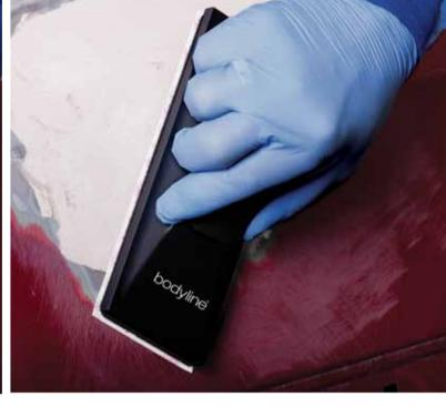
Final Flat Bodyfiller: Gripspeed Strips, P180 70 x 125, 70 x 198, 70 x 420, 115 x 228
