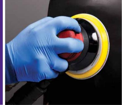
**Preparation Of Electro-Coat:** Gripspeed D.A. Discs, P320/P500 80mm, 125mm, 150mm
