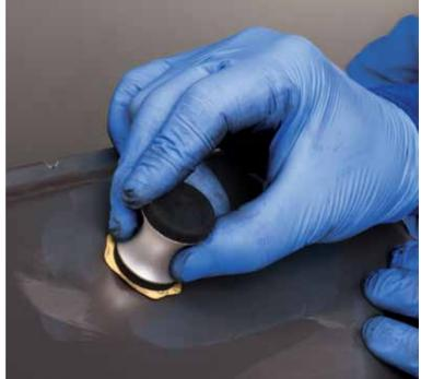
**Removal Of Minor Defects:** PSA Daisy Discs, P2000 35mm
