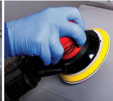
Final Flatting Of Primer: Gripspeed D.A. Discs, P500 80mm, 125mm, 150mm
