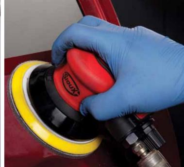
Blend Repair & Adjacent Panels: Gripspeed Blend & Finsh D.A. Discs or Gripspeed Film D.A. Discs, P1000 80mm, 125mm, 150mm
