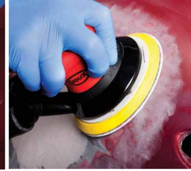
Feather Edge Repair: Gripspeed D.A. Discs, P180/P320 80mm, 125mm, 150mm
