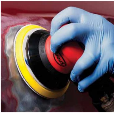
Preparation Of Damaged Area: Gripspeed D.A. Discs, P80 80mm, 125mm, 150mm
