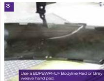
Apply Bodyline Plastic Cleaner BPC500 to the inside of the panel to remove all dirt and overspray from the damaged & surrounding area.
