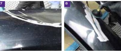
Create a shallow V next to the split Visual reference after the previous both inside and outside of the panel with a Bodyline Griplock Disc to provide
