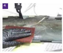
Abrade the area with a BDPBWPHUF Bodyline red or grey weave pad removing all dirt and overspray.
