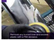
Sand the affected & surrounding area of the repair thoroughly with a Bodyline P180 grade disc BDPBSAD18015.
