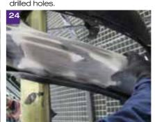
Finally, feather edge the surrounding area with P320 grade on a DA sander in preparation for following the recommended Paint process.
